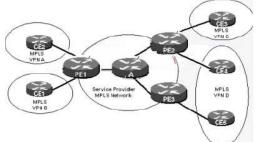
In the MPLS network shown, how many routing tables are on Router PE1?
