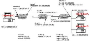
You work as a network engineer at Certkiller .com. With RIP running, what command would be used to set the default route on Router 2 to 171.68.64.6 (Router 3)?
