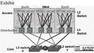
The diagram shows a campus with an L2 switched backbone. The backbone has a single VLAN (= subnet) with no loops. The links into the backbone are routed interfaces, not VLAN trunks. Switch X is the STP root of the core VLAN and switch Y is the standby root. The connection between X and Y is an EtherChannel. The network architect wants to add more redundancy by connection the L3 switches in the distribution layer to both X and Y. What best describes that plan?
