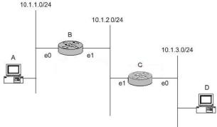
In this network, Host A is trying to reach Host D. There is no routing protocol running, but Router B and C have the following static routes configured: Router B: ip route 10.1.3.0 255.255.255.0 ethernet 1
