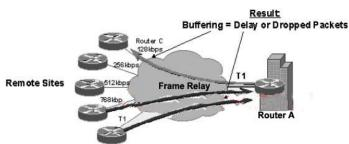
Examine the exhibit to view the topology. What mechanism should be employed to limit the "transmit rate" from Router A to Router C?
